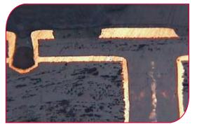
Buried via and applied SBU layer with blind via
