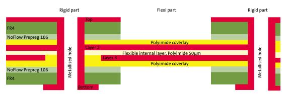
Abb. 2: Example structure of a 4 layer multilayer board with a flexible internal layer
