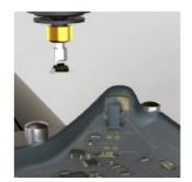
If the use of solder resist is necessary, there are two possibilities. On the one hand, before applying solder paste, solder stops can be selectively applied to sensitive areas using a separate processing head of the auto-
