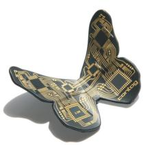
possibilities that can only be realized in the overall system by MID in a technologically sensible and cost-effective manner. Here 3D-MID offers the intelligent and elegant solution of system development. CONTAG offers a comprehensive service for 3D-MID projects, from consulting in the design and selection of a suitable material through rapid prototyping to series production and assembly.
